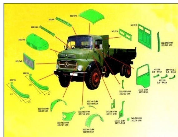
Fig5. Different parts of ECE-R29 truck cabin
