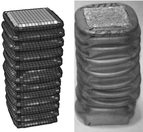
Fig5.. Comparison of experimental deformation [22] with numerical prediction.
