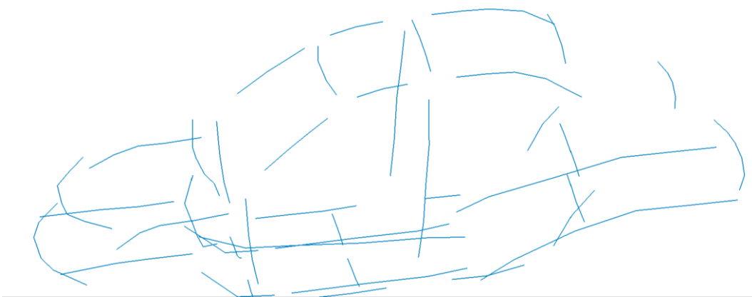
Fig3.: Equivalent beam modeling of the BIW
