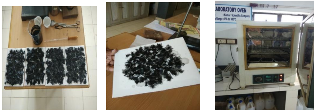
Fig 2.5 Grafting MWCNT-F on CF Surface
