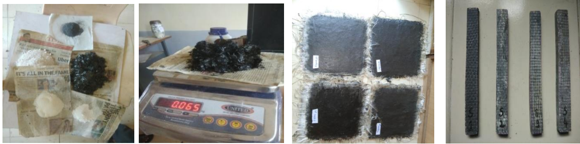
Fig 3. Sequence of operations carried in fabrication of composite sheets
