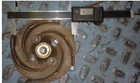
Figure 3: View of the pump's impeller
