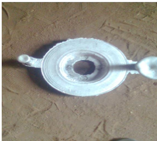
Figure 7: Aluminium Based alloy automobile brake disc with 25%SiC reinforcement particles after casting
